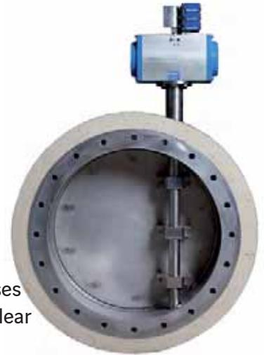
Unlike dampers with an “intumescent seal”, the damper is mechanically sealed via a system of flaps and specially-machined reverse-slope seats that are fitted to the tunnel body using a high-precision joining process.
